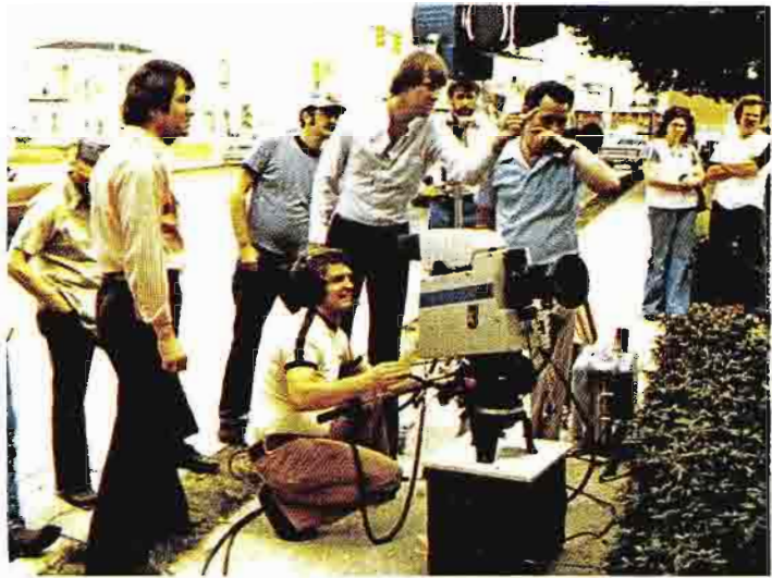
TK-760 rides comfortably on short mount, with a viewing receiver as a base.
