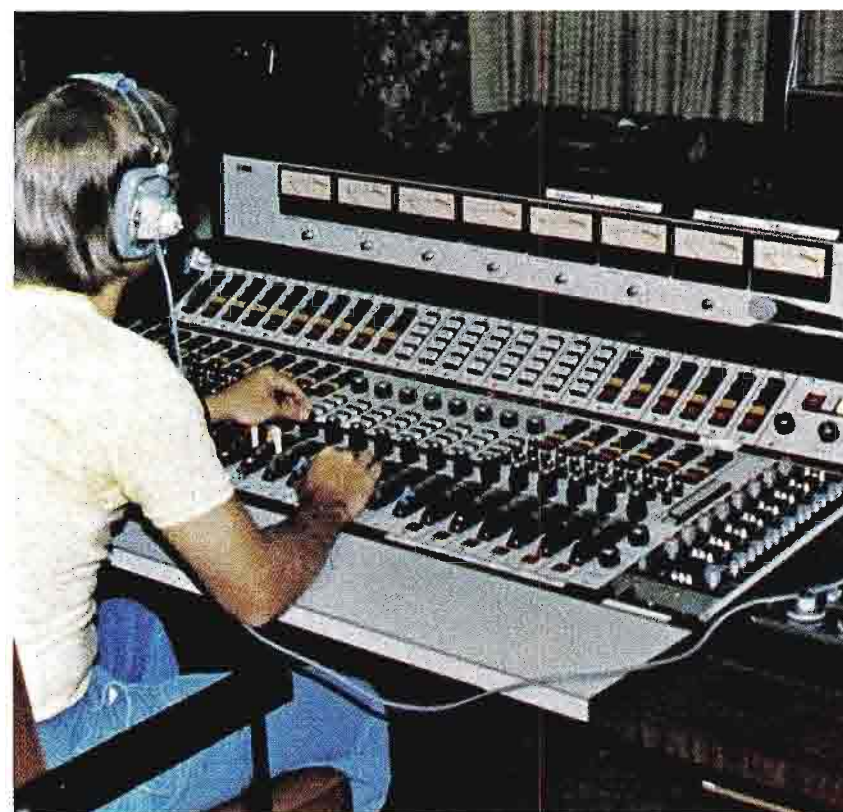
The RCA BC-100 audio board gets a run-through by an ORU Telecommunications student.
