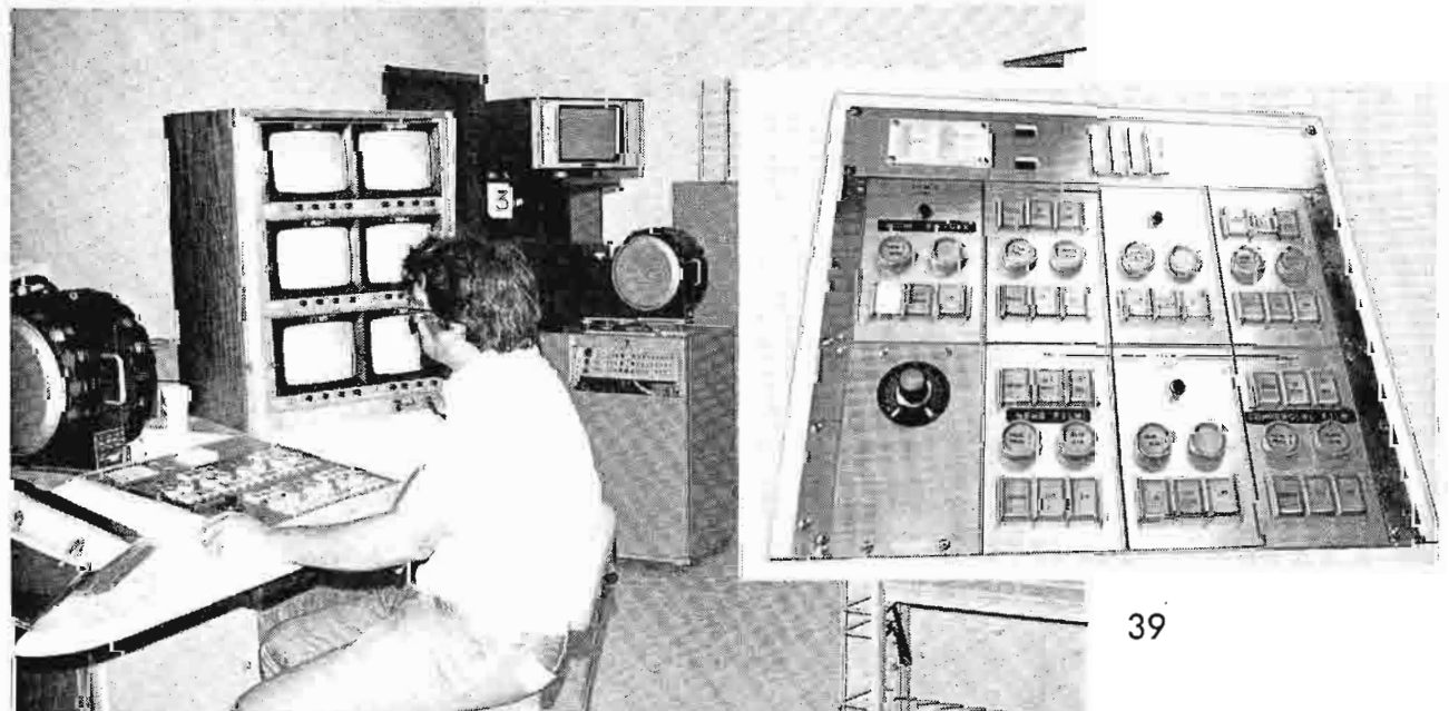
KMTV-designed remote telecine machine panel (inset) and bank of monitors aid in production and on-air operations.
