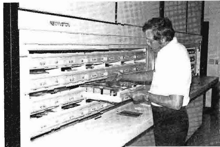
Computerized retrieval system in Media Dept. offers instant access to video "carts" and film spots.
