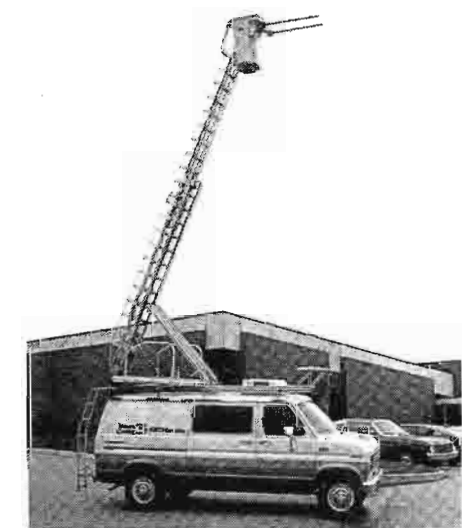
The KMTV ENG complement includes a microwave-equipped van for extended distance direct transmission to the studio.
