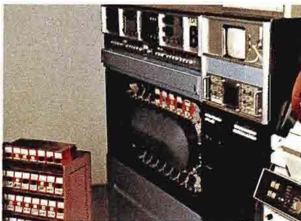
Technical area at CKY includes two TCR-100 video "cart" machines; two-600A VTR's with AE-600 Time Code Editing Systems, and a new TK-28 Telecine system.
