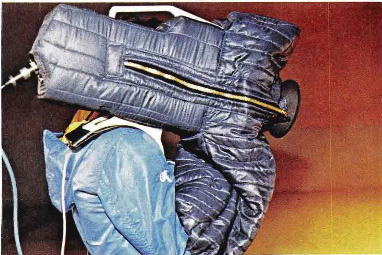
In deference to the severe weather conditions, CKY had special cold weather jackets made up for their TK-76 and TK-760 cameras.
