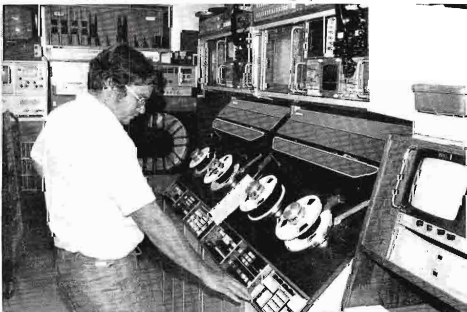
Tape production is handled by TR-600A VTR's equipped with AE-600 Time Code Editing Systems.
