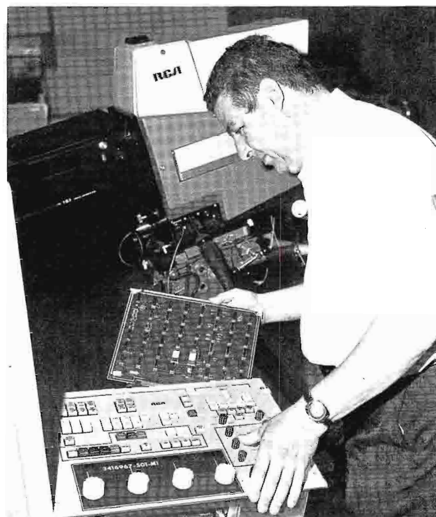
Two plug-in modules are added to the TK-47 Set-up Terminal for fully automatic camera set-up capability. RCA Broadcast Systems engineer Robert A. Dischert (photo) has been awarded a U. S. patent for the automatic set-up system.
